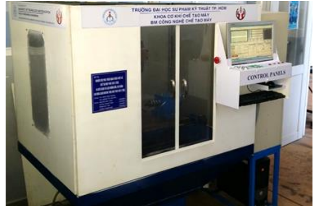
Figure 10. 2: A 5-axis CNC milling machine capstone project
